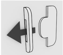
4. Add the remainder of the tab holders (9) (E) to back of the base into the slots as image below.
