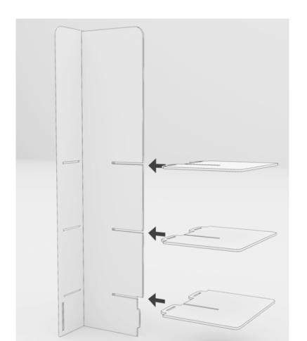
3. Bend the flaps of base bottom (D) align tabs into back of base (B) add tab holders (2) (E) as shown below to slots.
